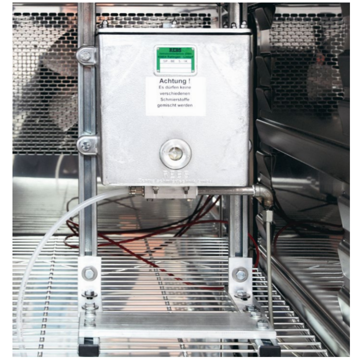
Test bench for wheel flange lubrication
