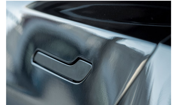
Door handles optimized for minimal wind resistance: Hydrophobic coatings can reduce the disruptive influence of water
