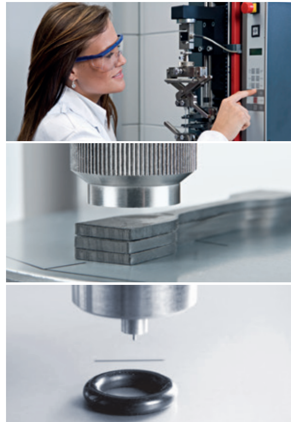
Tensile strength test (upper picture) and hardness tests of elastomers
